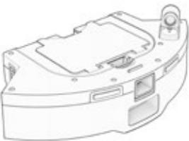
3. Align the mop attachment connectors with the dustbin's and press to lock in place.
