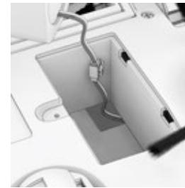
3. Slide the new battery into UltraVision.
