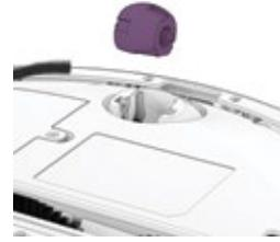
2. Once the wheel is removed, use the screwdriver to pry out the wheel assembly.
